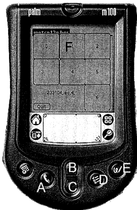
Figure 1 – A Palm M100 handheld computer running METEORCOUNT. Explanations are in the text. A Leonid of magnitude +4 has been entered at 23^{\text{h}}31^{\text{m}}04^{\text{s}} by simply hitting field (F) 4. The keys A, B, C, D, and E allow more complicated entries, as explained in the text.
